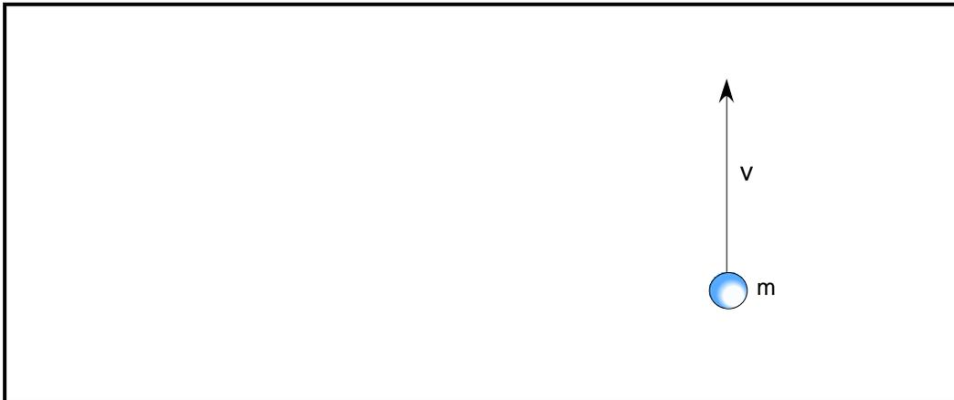
In space (in a vacuum), the blue body moves at a constant speed  $v$  in the same direction. Without an exogenous force, the body retains its original speed  $v$ . (Newton's First Law of Motion)
